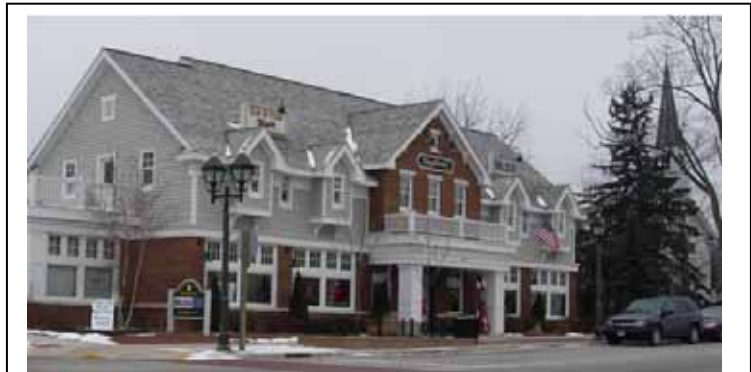
Figure 17—Facades that face public streets or adjacent development shall be subdivided and proportioned using features such as windows, entrances, arcades, arbors, awnings, trellises with vines, along no less than 60% of the façade.
