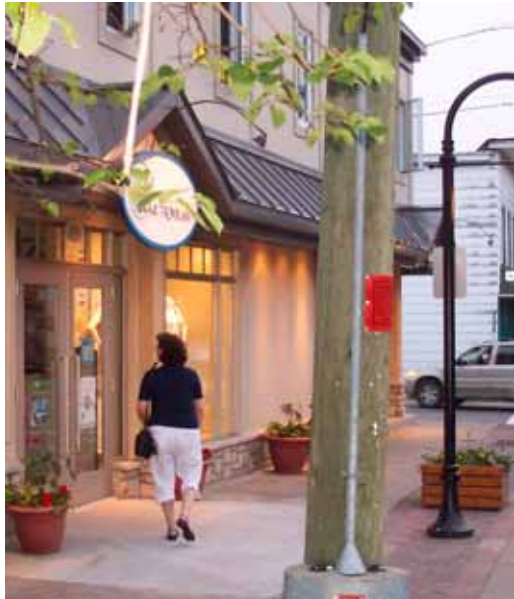
Figure 13—On-site pedestrian walkways shall connect each primary entrance of a commercial building to the adjacent parking blocks, structures, or site amenities.
