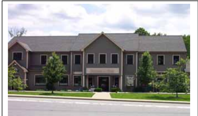
Figure 16— No wall that faces a street or connecting pedestrian walkway shall have a blank, uninterrupted length exceeding thirty (30) feet without including architectural features such as columns, ribs, pilasters or piers, changes in plane, changes in texture or masonry pattern, or an equivalent element that subdivides the wall into human scale proportions.
